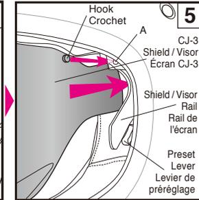
When the shield/visor rail goes into the gap between the shell and the liner (the shield/visor housing space) like Drawing A, insert a tool such as a flat-head screwdriver covered with soft cloth into the shield/visor housing area and get the shield/visor rail down.
