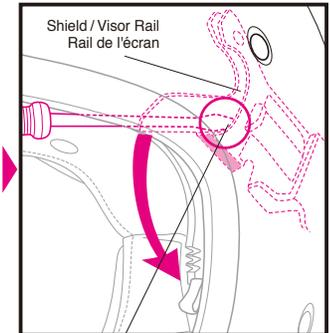
The Shield / Visor Housing Area of Shield / Visor Rail
