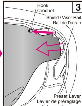
**!** Do not leave the preset lever in the position 0 (the lower position than the position 1). The lever may be deformed.
