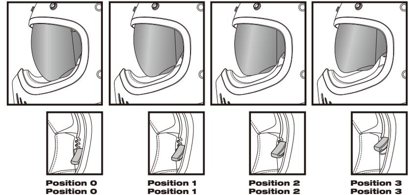
For changing height of the preset lever, open a shield / visor, push the preset lever to outside slightly and move it to the gear of the required position.
