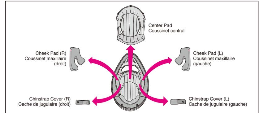
The center pad, the right and left cheek pads and chinstrap covers can be removed for washing. You can also adjust the fit of your helmet by switching to the optional pads. Look at the list and drawing of interior parts and check whether the parts are installed or removed. Be sure to always fix the center pad, cheek pads, and chinstrap covers prior to riding. If necessary, use the following table to order the proper interior parts to adjust the fit of your helmet.
